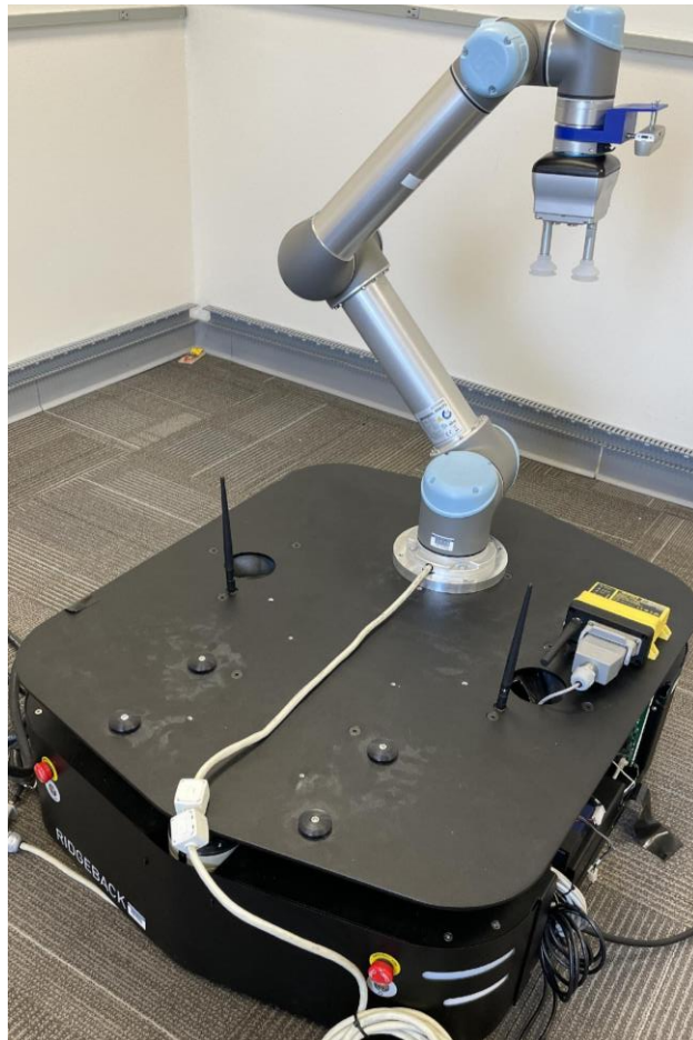
Figure 11. Photo of the final Ridgeback™ with UR5 system.
